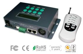
LT-800 DMX512 controller is the output signal of international standard DMX512/1990. It not only can control all the LED lights that receiving the standard DMX signal in the market, but also can work with our DMX decoder to control the general LED lights without DMX512.
