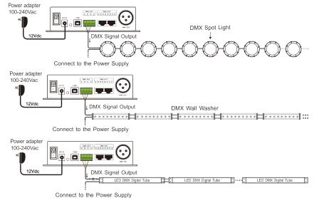
[Attn] Please confirm the LED lamp can receive standard DMX512 signal, otherwise it can't work properly.
